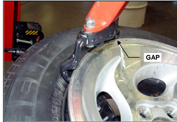
INCORRECT (NOT FULLY SEATED) MOUNT/DEMOUNT HEAD
